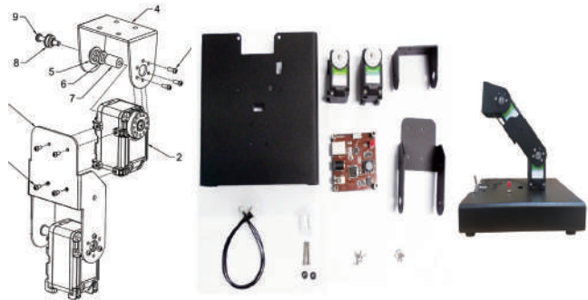
[2-Axis Manipulator Disassembling and Assembly Practice]
