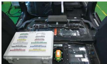
Battery part cutting and check terminal
